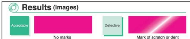
**Fig 6: Check for Scratches or Dents**
